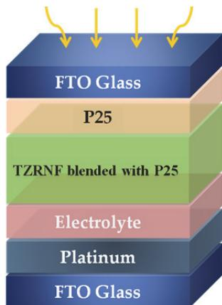
**Fig. 1 Schematic diagram of the DSSC developed in this study**
