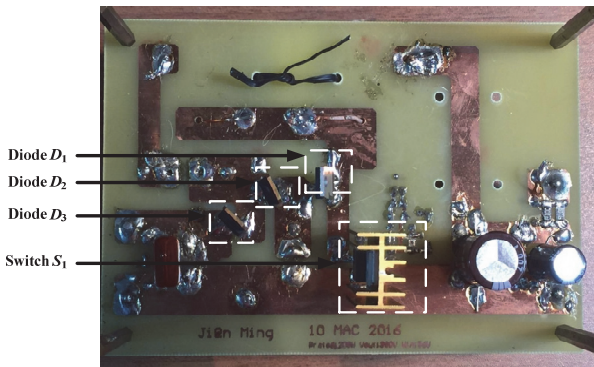
Fig. 43 Reverse side of the prototype circuit.
