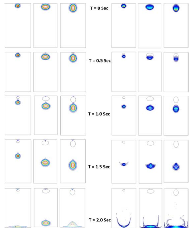
Fig. 6 Viscosity Distribution of spherical and spheroidal Carreau model fluid droplets of n=0.4 settling in stagnant air a) Spherical b) Oblate ellipsoid c) prolate ellipsoid
