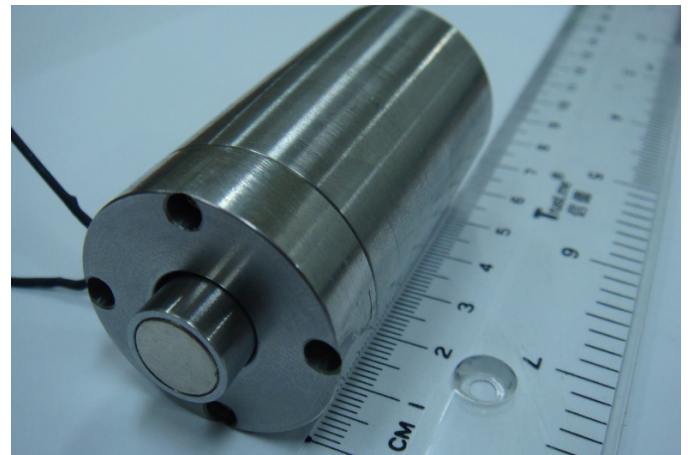
Fig. 12 Photograph of the realized prototype of linear motor.
