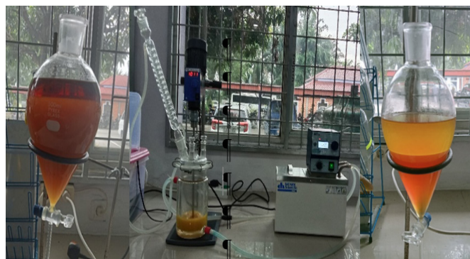
Fig. 4 Esterification and transesterification process
