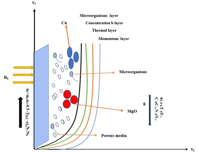
Fig. 1 Flow structure of the physical MHD-HNF model
