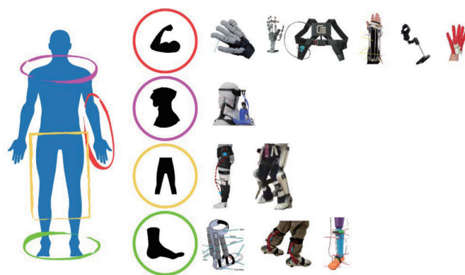
Fig 4 Diagram of the human body showing the areas assisted using various soft actuators as per the reference article.
